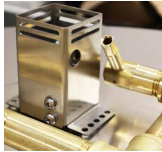
Photo 4b: Pilot Hood Circular Opening Positioning
