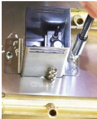
Photo 5: Securing the Pilot to the Plate/Pan
