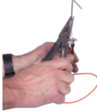
Figure 9: Fixing the Electrode
