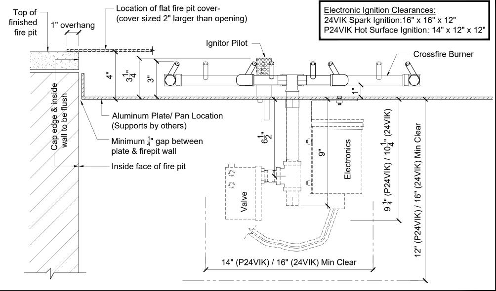
Dwg: S:\ AutoCad Drawings\Critical dimensions
