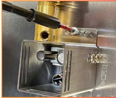
Photo 5: Securing the Wind Cage to the Plate/Pan
