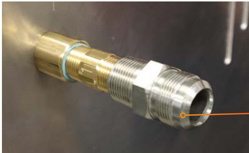
Photo 17: Attaching the Male Flare Hose Adapter
