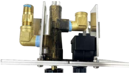
Photo 8b: Applying Joint Compound
